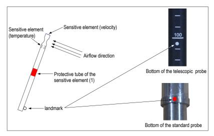
Before any use of the device with an air velocity probe, please lower the protective tube (1) of the sensitive element (except vane probe).
